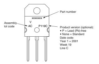
Example: This is a xxxxxxx with assembly lot code AC, assembled on WW 19, 2001 in the assembly line "C"
